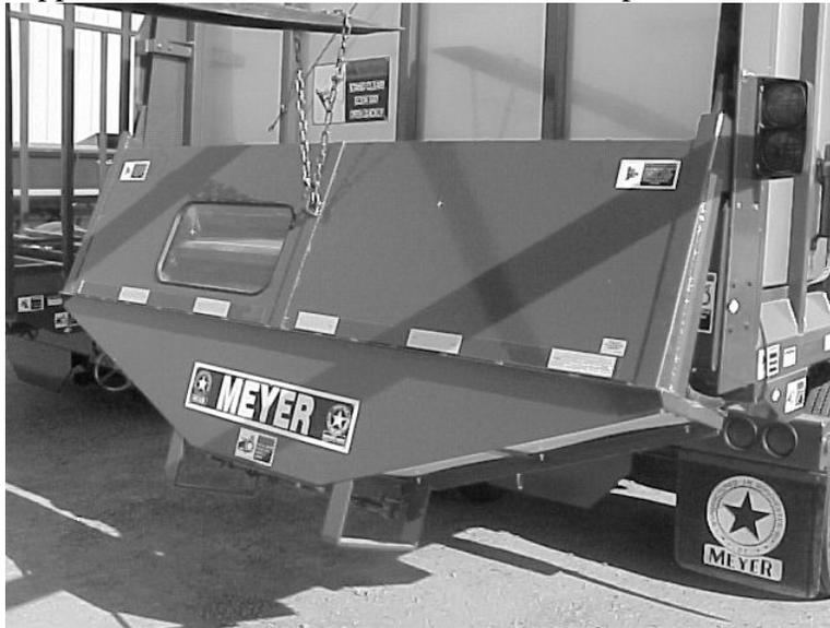
After the grain hopper is in place tighten the turn arms under the back side of the implement to pull the hopper tight to rear of the box. (See Below)
