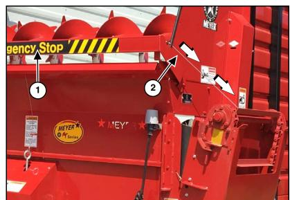
NOTE: The emergency stop mechanism DOES NOT STOP rear unloading operation of the forage box.
