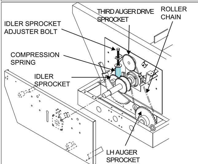
**FIGURE 11. LH & THIRD AUGER CHAIN DRIVE**
