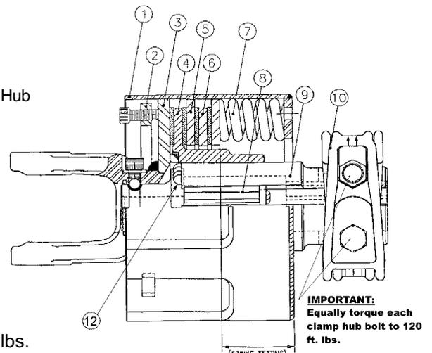
**\*IMPORTANT:** Equally torque each clamp hub bolt to 120 ft. lbs.
