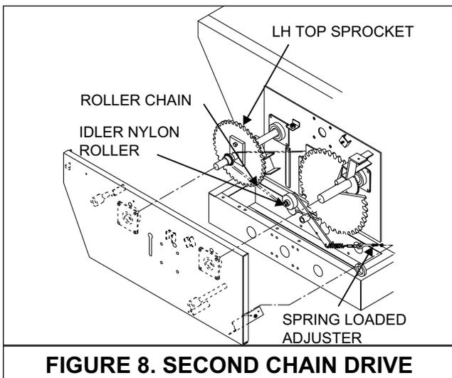
The second chain drive (large RH top sprocket to the large LH top sprocket, figure 8) is automatically tensioned by a spring loaded idler nylon roller. The extension spring should extend 3/4" from its neutral 4" total length.
