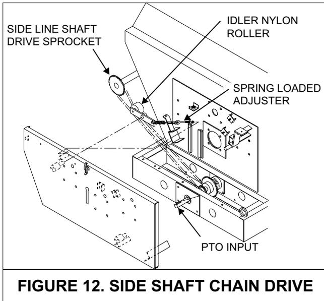
The side shaft chain drive (PTO input shaft to the side line shaft drive sprocket, figure 12) is automatically tensioned by a spring loaded idler nylon roller. The extension spring should extend 3/4" from its neutral 4" total length.
