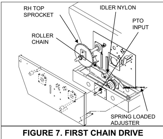
The first chain drive (PTO input shaft to the large RH top sprocket, figure 7) is automatically tensioned by a spring loaded idler nylon roller. The extension spring should extend 3/4" from its neutral 4" total length.
