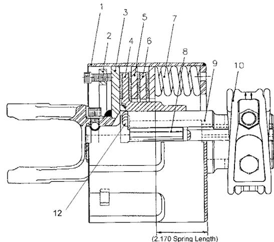
**\*IMPORTANT:** Equally torque each clamp hub bolt to 120 ft. lbs.
