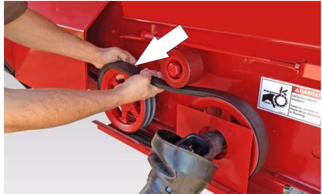
9. Move the Independent Outfeed Clutch control lever (Item 1) to "RUN" (down). Check for proper tension. Adjust as needed. (See Independent Outfeed Clutch Adjustment).
