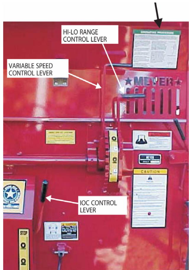
Three levers control operating the front unloading unit of the forage box.
