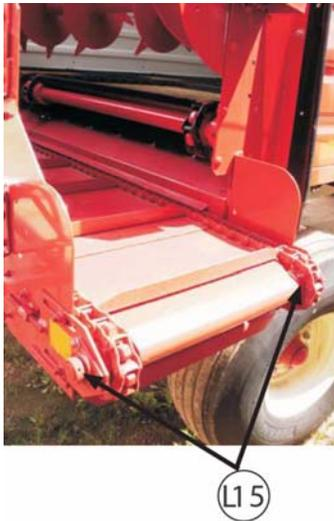
(A1) Adjust main apron chain per “Adjustments” section. Adjust cross conveyor chain per “Adjustments” section.
