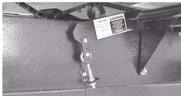
**PRIOR TO 08 SERIAL NUMBERS** - To tighten the main aprons, tighten down the anchoring eye bolts centrally located at each side of the forage box on the steel 10" stringers.
