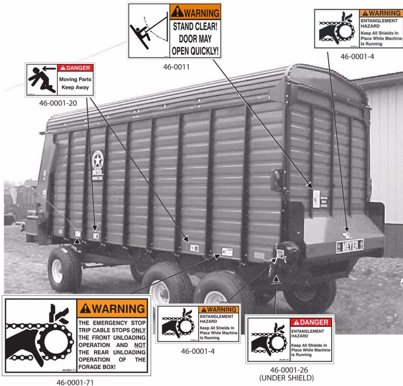
**! CAUTION: READ ALL DECALS ON THE FORAGE BOX AND IN THIS MANUAL. KEEP THESE DECALS CLEAN AND REPLACE ANY LOST OR DESTROYED DECALS. BECOME FAMILIAR WITH ALL TRACTOR AND FORAGE BOX CONTROLS.**
