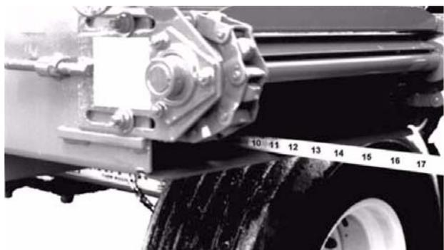
Correct adjustment of the cross apron chain occurs when 12" of chain, APRON SLAT does not touch the BOTTOM PAN of the cross apron return area at the discharge opening. To tighten the chain, loosen the two bolts securing the slotted bearing bracket at each side of the discharge opening. Tighten the chain by tightening the nut on the adjuster bolt. Adjust both sides equally. Retighten the bearing bracket bolts.
