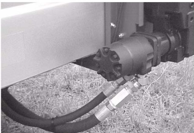
**HYDRAULIC CHECK VALVE AT REAR OF BOX**
