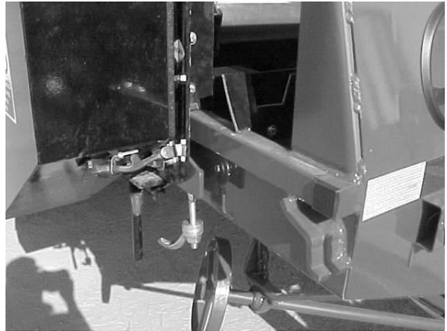
Once grain kit is started into receivers, simply slide the grain kit up tight to the back of the box. Tighten the turnbuckles into the slotted clamp brackets on each rear corner on each side and draw grain kit up tight.
