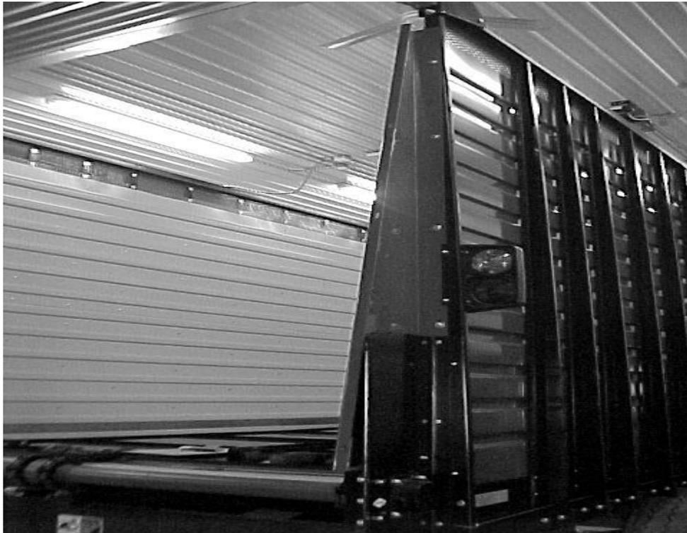
Drill 13/32" diameter hole on inside bottom corner and bolt tight using 3/8 x 2" machine bolt and 3/8" spin locknut. Do not over tighten. (See photo below.)
