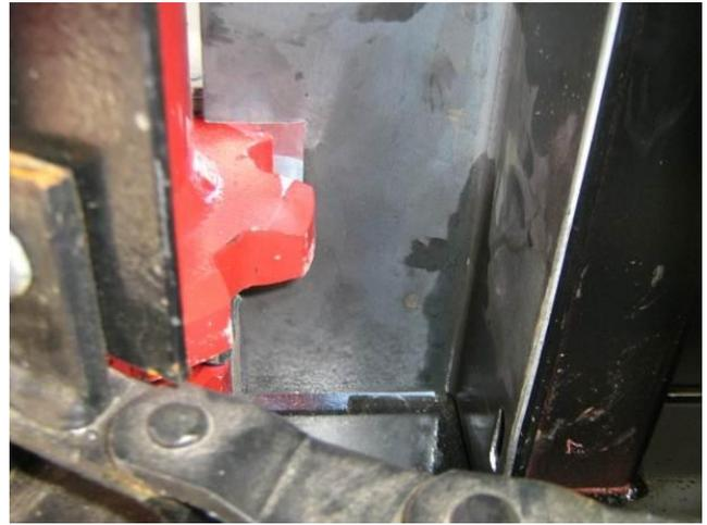
Tighten the nut enough so the bolt can turn freely. This will allow the bolt to move in the slot if the poly floor expands/contracts.
