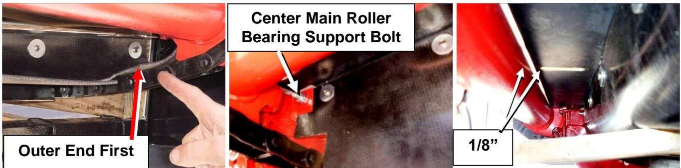
Insert the side toward the outside of the box first. Next slide the side toward the center in lifting up and around the center main roller bearing support bracket bolt. Then slide the whole assembly back toward the main roller so that there is a 1/8" gap between the main roller and the seal kit plate. Clamp to hold in place.
