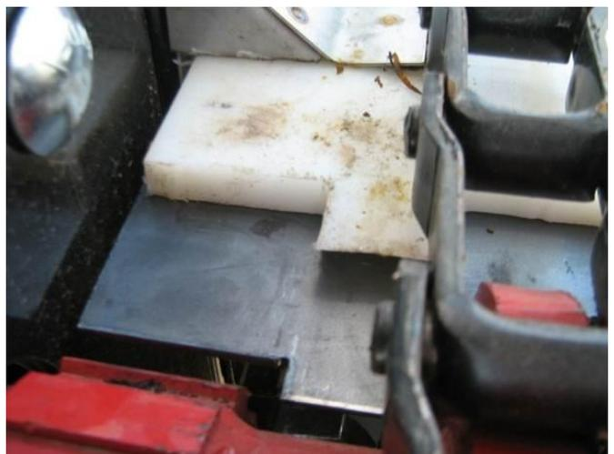
Once the metal floor pieces are fully secured, locate two longer slots in each metal piece that run the length of the box. With a drill bit, drill a hole in the poly floor, centered in each of the four total slots. Insert one 5/16" stainless truss head machine screw in each hole and place a washer on the bottom side, along with an indented locknut.
