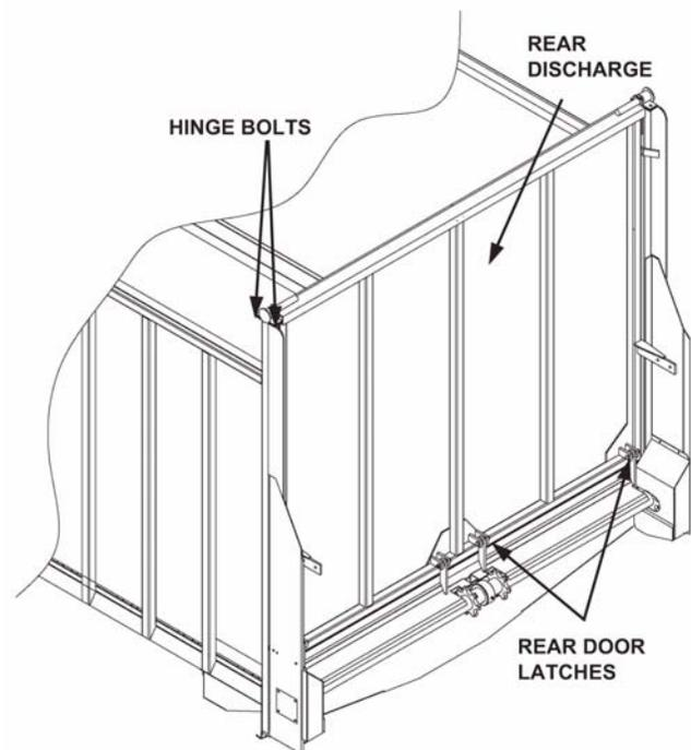
**FIGURE 2. REAR OPENING DISCHARGE DOOR
