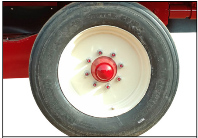
Figure 8.30 Grease Lubricated Wheel Hub
