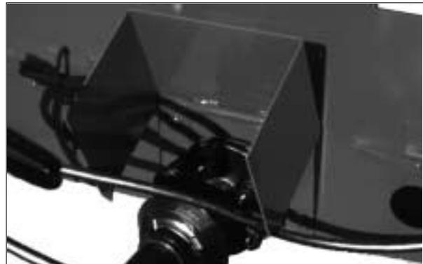
FIGURE 7. PTO SHIELD FLIPPED UP
