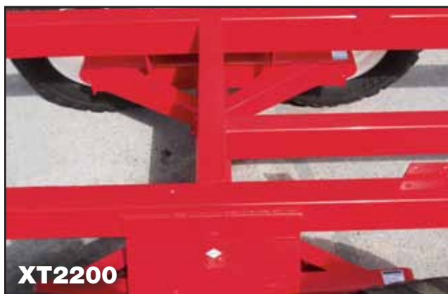
XTSS2200XL Suspension axle with rear steer
