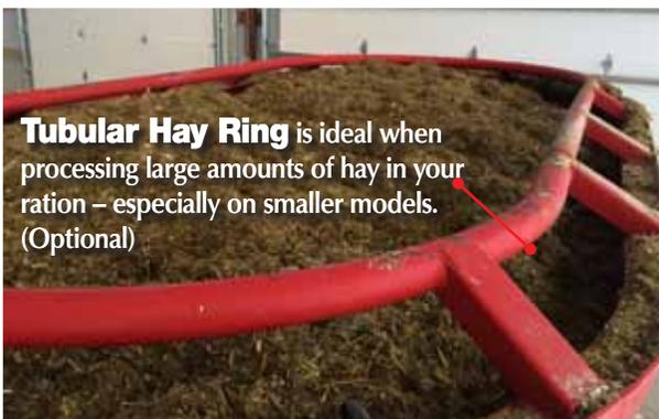
**Tubular Hay Ring** is ideal when processing large amounts of hay in your ration – especially on smaller models. (Optional)
